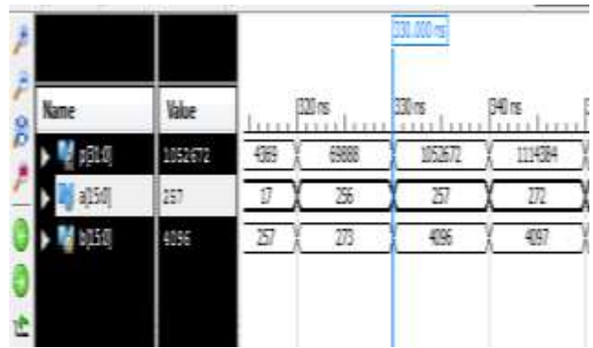
Fig13. Simulation Result of 16 Bit Column Bypassing Based Braun Multiplier with KSA
