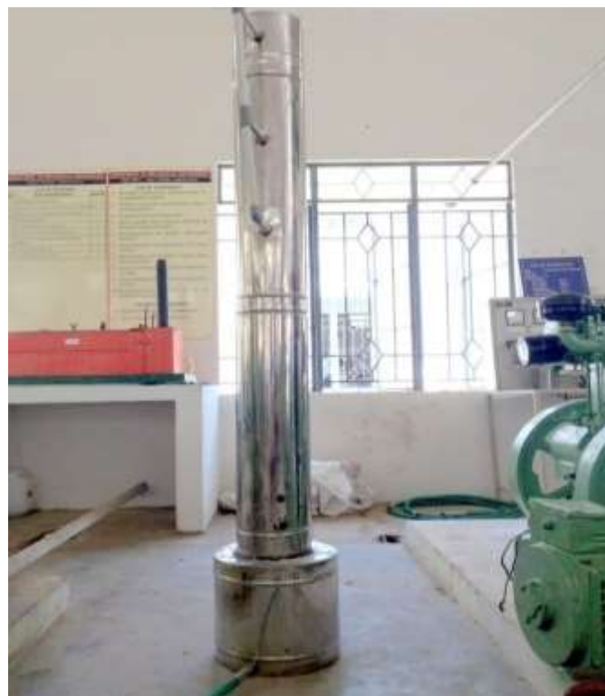
Fig. 1 Dual type scrubber setup
