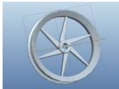
figure 1.1 3d model of alloy wheel created by using pro e
