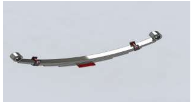
Figure 8.1 Leaf spring models
