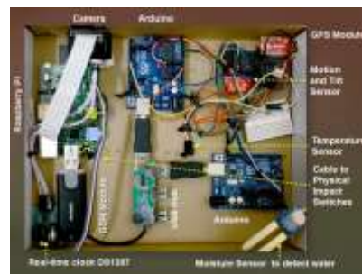
Figure. Image showing our Black Box prototype & its components.
