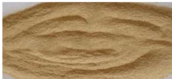
Figure3.5 Fine powder form Briquettes from rice straw
