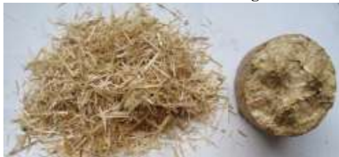
Figure3.4 Briquettes from wheat straw
