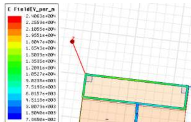
Fig. 3 Electric field under Excavated coupling element
