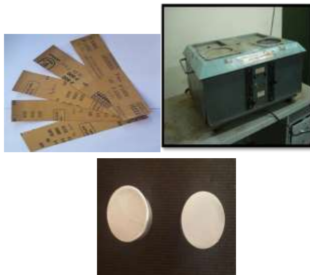
Figure 2: Depicting the images of emery paper, polishing machine and polished specimen for microstructure
