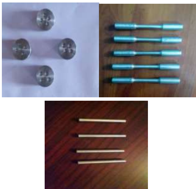
Figure 3: Depicting the images of Hardness, Tensile and Wear Test samples
