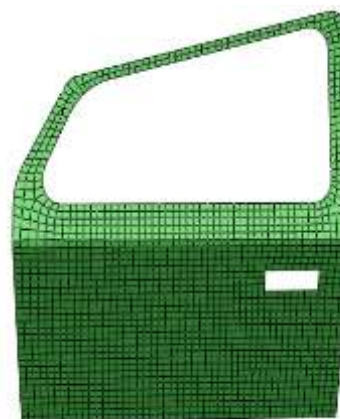
Figure 2: meshed car door model.
