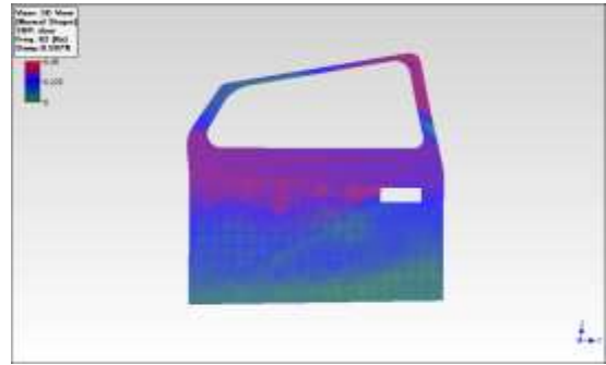
Figure 9: 8 th Mode Shape And Frequency Is 62 Hz In Free-Free Condition Without Damper.
