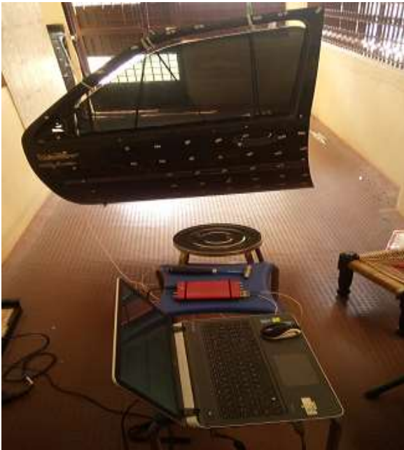
Figure 7: Shows The Experimental setup Of Car Door.
