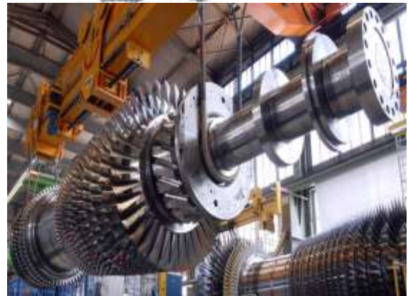
Gas turbine application for power generation
