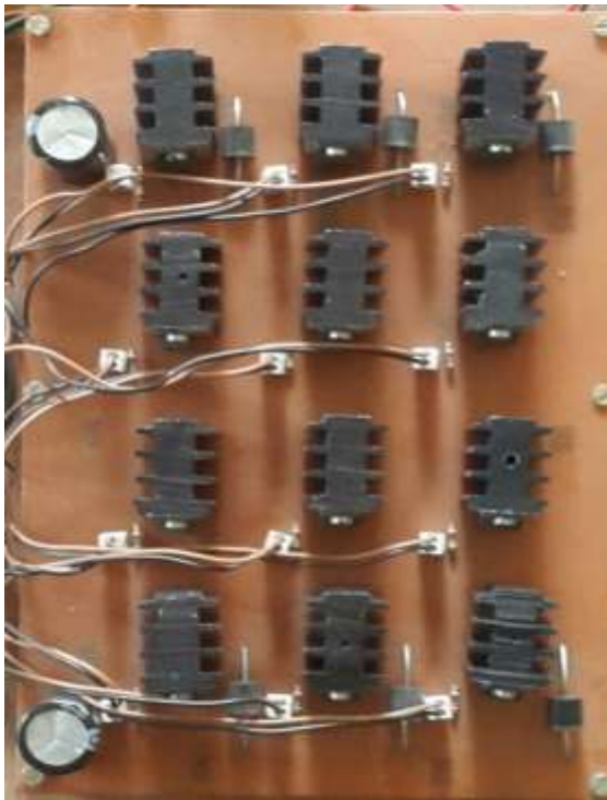
Fig. 2. Multilevel inverter based drive circuit.
