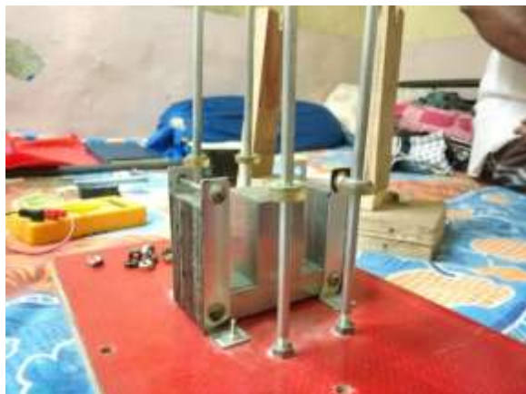
Guidance Mechanism using Four Bolts (Bottom)
