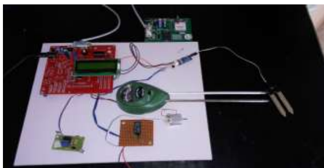
Fig 12 Hardware Setup of Maize Monitoring
