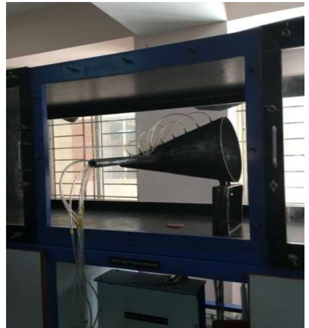
Model mounted inside the wind tunnel and connected to water manometer through pressure ports.
