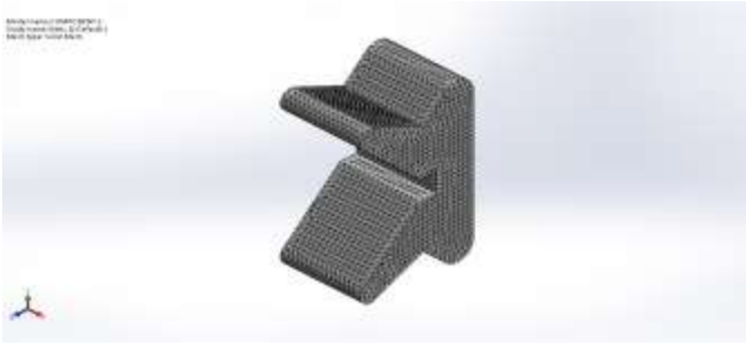
Fig 4. Meshing of Punch
