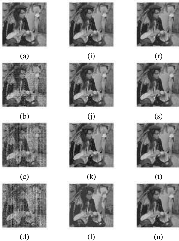
Fig. 11: Reconstructed benchmark image [13, 14] for varying ET using BWA-DCT (a-d), TEA-DCT (i-l), and proposed DCT (r-u) architectures.
