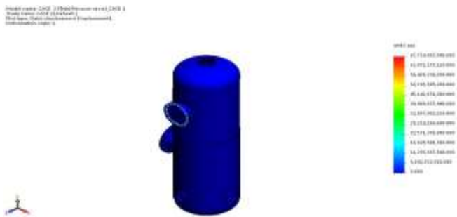
Fig 1.2 static displacement (pressure vessel) in simulation
