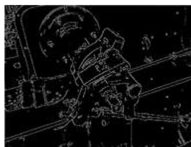
Fig. 13 Image after applying canny edge operator[13].
