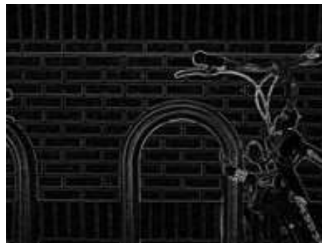
Fig. 11 Image after applying prewitt operator[12]
