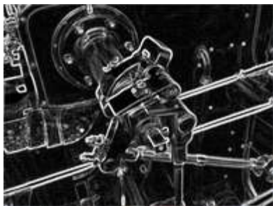
Fig. 9 Image after applying sobel operator[11]
