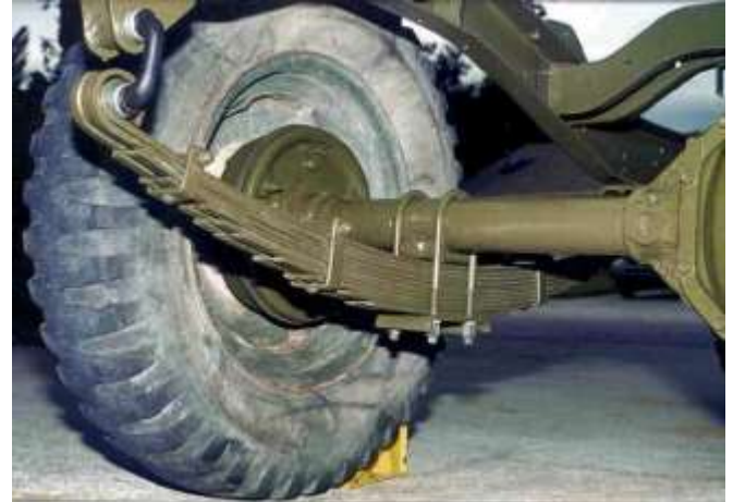
Fig.1 Leaf spring assembled at rear axle of automotive
