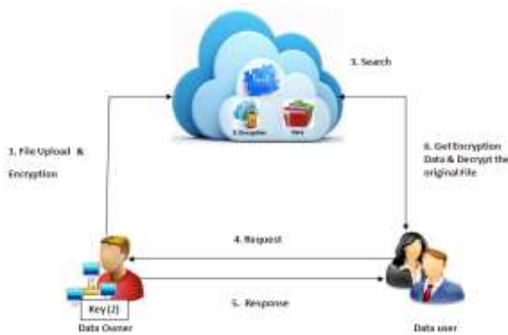
(a)The Architecture of Dual Encryption Scheme and Automatic key Generation over cloud data.
