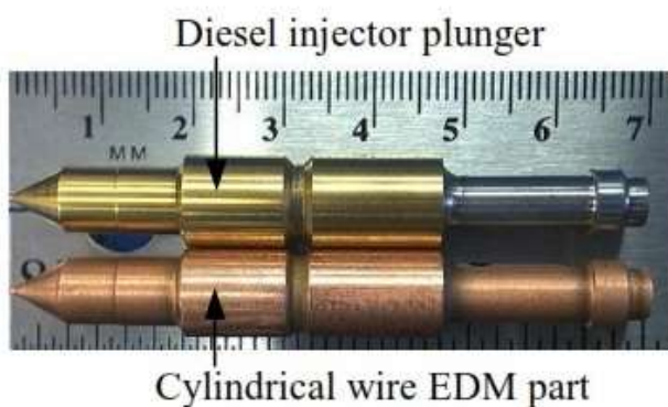
Fig 3: A cylindrical wire EDM part with the same shape as the diesel engine injector plunger [10]
