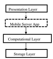
In the figure above Mobile Server Application as if it is the fourth layer of communication, which is seemingly true because the whole storage and CPU of the system is at the VMS server hence each clients hosted MSA is behaving as a visual API between two end devices; but it will work much faster than the web server as all the resources and computations are stored at a same place.
