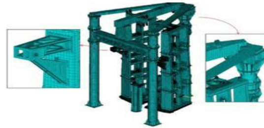
Fig.2 FE model of the sector Sub- assembly Tool.
