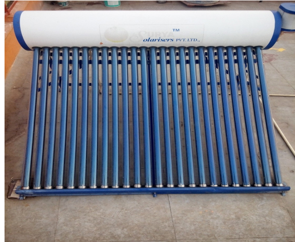
Fig.1 Experimental set up of 200lts solar water heater
