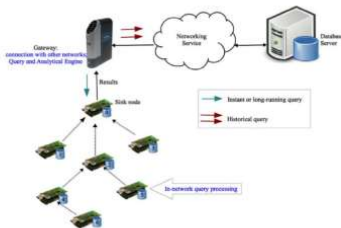
Fig. 2. Illustration of a distributed database architecture for wireless sensor networks
