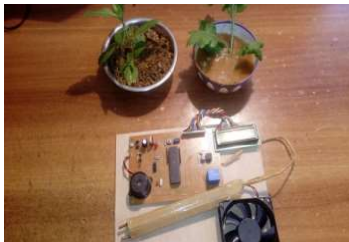
Fig: 8.1 prototype of the Automatic Irrigation System
