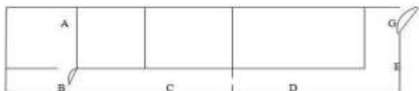
Fig 9: Node position for coverage range test inside the building
