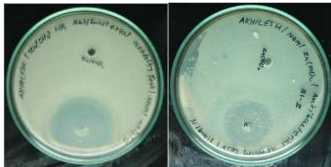
Fig.:2- The inhibited zones of bacterial growth shown by Zinc Hydroxide NPs
