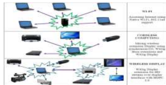
Fig1. Inter-communication of Wi-Fi
