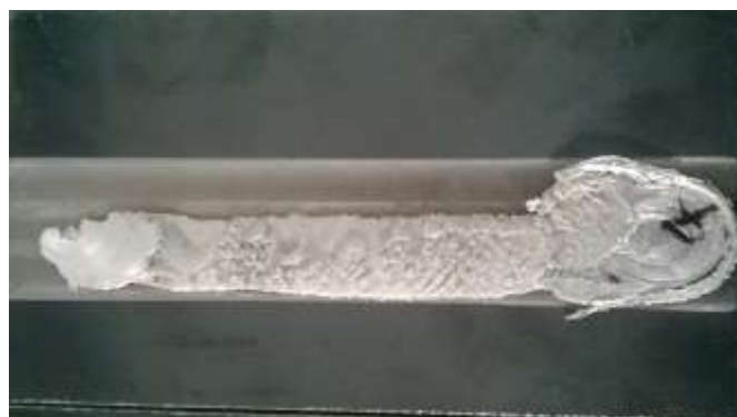
Fig.2. After coating of AA 5083 over Mild steel and the formation of layers along the plate
