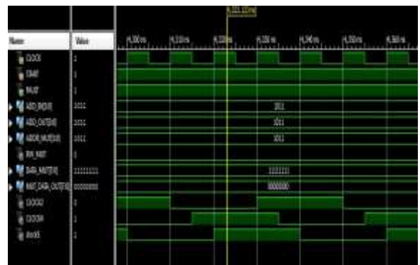
Fig.13: Waveform found faulty on reading 1 at 1011
