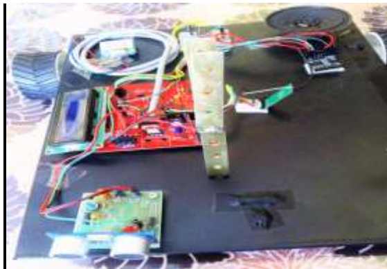
Fig. 7 Robot unit with an ultrasonic sensor and controller
