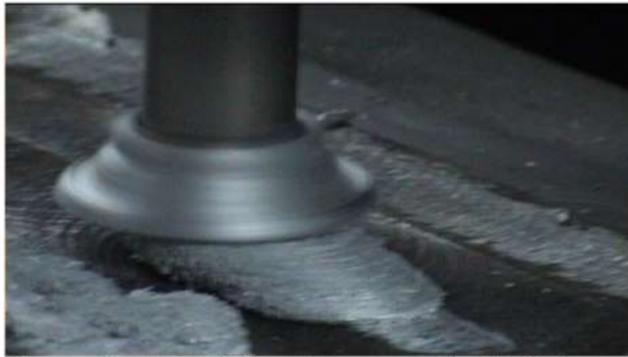
Fig.3 : Coating of Aluminium over the M.S.plate
