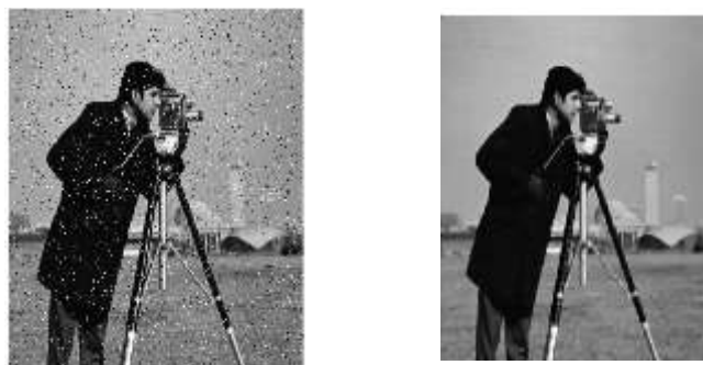
(a) Input to median filter (b) Output from median filter
