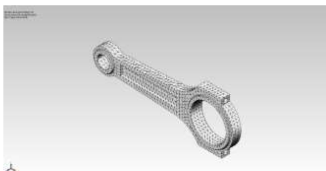
Fig. 2 Meshed connecting rod
