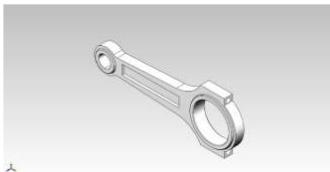
Fig. 1 Solid model of the connecting rod
